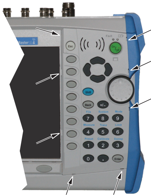
Location of the 8 tabs holding the keypad bezel
